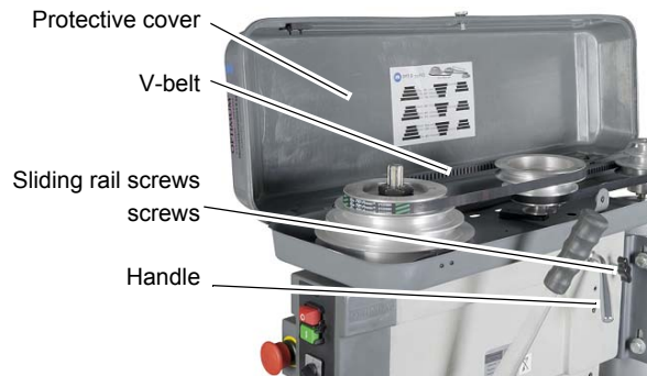
Img.4-4: Belt drive
