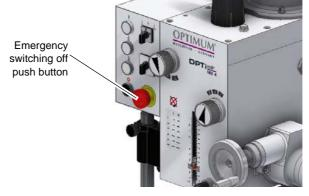
Img.1-2: Emergency switching off push button
