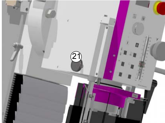
Img.4-4: Mechanical securing, quick clamping system
